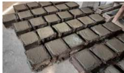
Figure 1- Casting of Specimens
